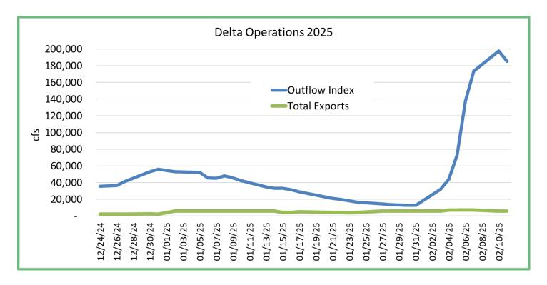
The anomaly was driven by two factors. First, a restriction on flows heading to the pumps. To protect endangered fish, flows toward the State and Federal pumps are capped at 5,000 cfs during the first half of the year. During very wet periods this restriction is not necessarily limiting because the San Joaquin flows are usually high, and the pumps can operate at their permitted capacity by pumping San Joaquin
